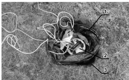
Fig. 3. Arrangement of temporary point of seismological observations: a) installation of seismological device in the ground (1 - waterproof material, 2 - seismological device, 3 - deepening), b) installation of seismological device at building levels.
