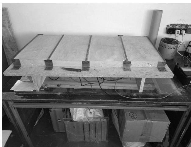
Fig. 3. An example of the disposition of the heating panel for floor heating simulation
