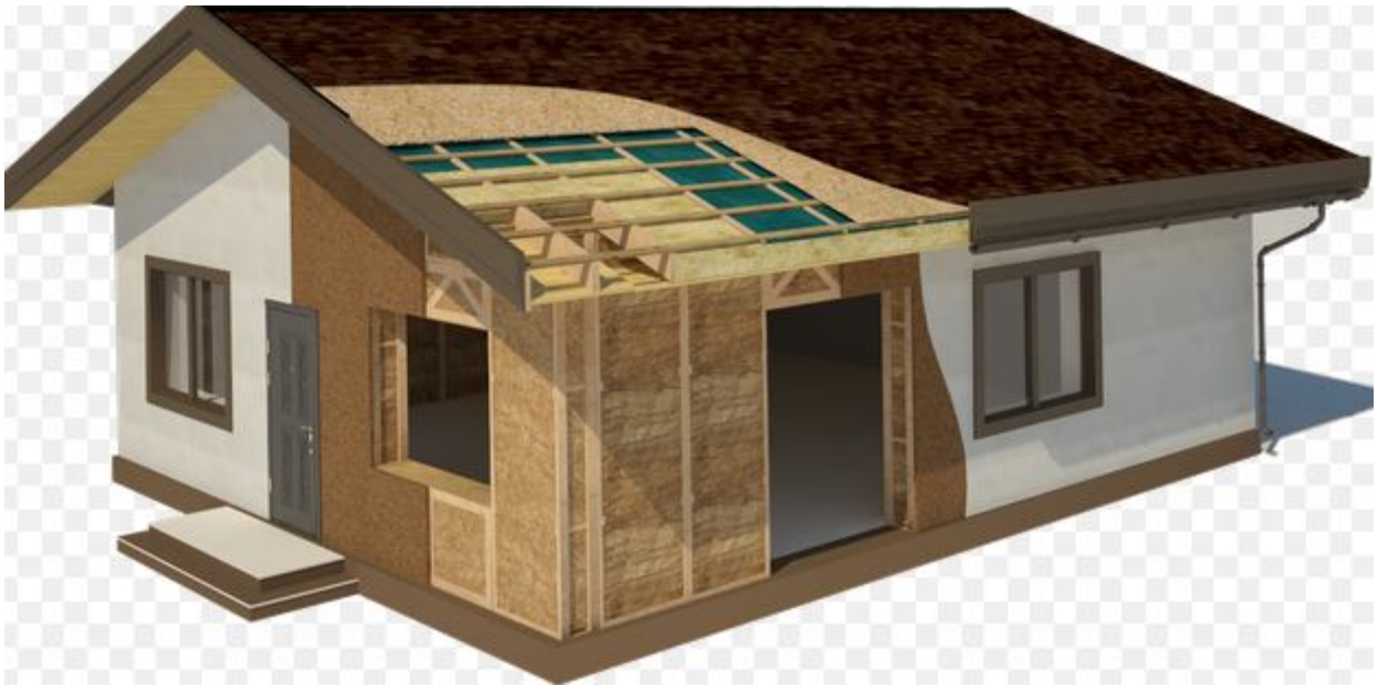
Fig.1. The design of the house using straw panels
