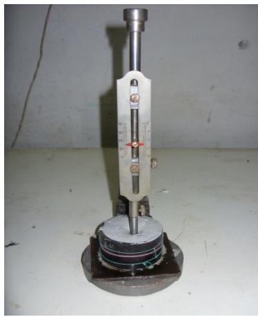
Fig. 1. Testing the standard consistence a) and setting time b) of concrete
