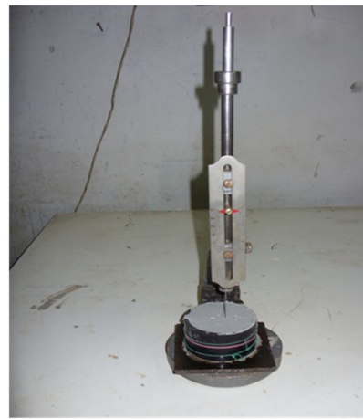
Fig. 1. Testing the standard consistence a) and setting time b) of concrete
