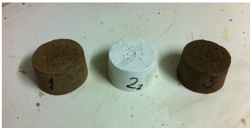
Fig 2. The general view of the specimens of compositions 1-3 after determining the setting time
