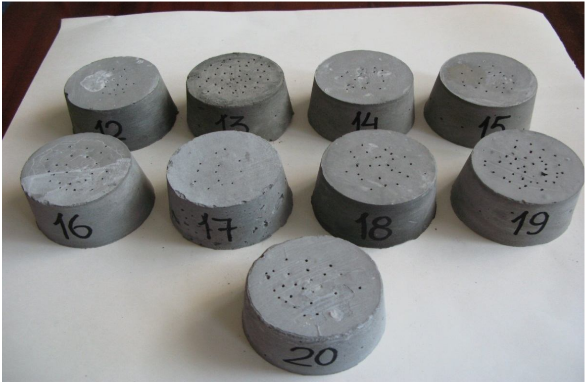
Fig 4. The general view of the specimens of compositions 12-20 after determining the setting time
