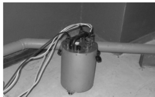
Fig. 3. Arrangement of temporary point of seismological observations: a) installation of seismological device in the ground (1 - waterproof material, 2 - seismological device, 3 - deepening), b) installation of seismological device at building levels.
