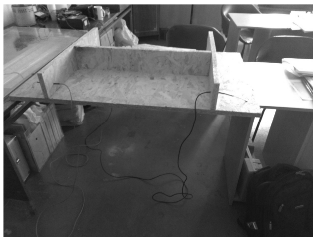
Fig. 5. An example of the disposition of the heating panel for the ceiling heating simulation
