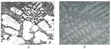
Fig. The microstructure of alloy Al4S before and after modification: a – before modifying  $\times$  400; b – after modification  $\times$  400
