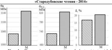
**Fig. 1.** The mechanical properties of heat-resistant nickel alloy XH59MBTKIOJ before and after modifying (M - modified alloy).
