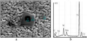
Fig. 3. The microstructure of the modified nickel alloy XH59MBTKIOJI, x 15000 (a), and the schedule of the intensity distribution of the characteristic radiation of elements (b).
