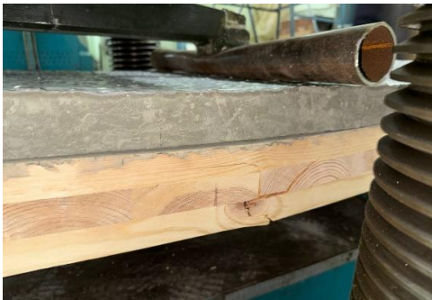
Fig. 1. Failure pattern of RAC-CLT panel
