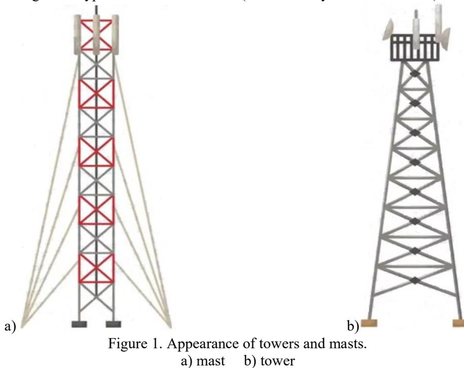
Figure 1. Appearance of towers and masts.
