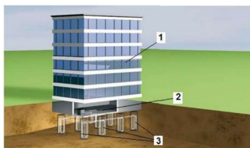
Fig. 2. The general layout of the building's elements heated with the use of energy piles: 1 – heated building; 2 – technical basement with heat pumps; 3 – energy piles with heat pump collectors
