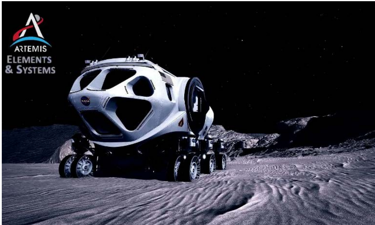
Fig. 1.8. NASA Habitable Mobility Platform based on the post Constellation Space Exploration Vehicle.
