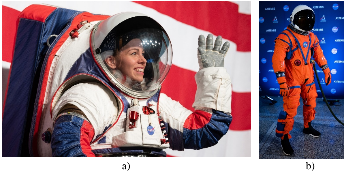
Fig. 1.10. Suit: a) xEMU suit for lunar surface extravehicular activity (EVA); b) OCSS suit for launch and reentry
